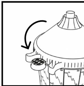
The sturdy and ergonomically shaped DrehFix pegs ensure easy and secure screwing on and off of the lid without squeezing the cup.
