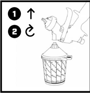
Attach the cup by gently pressing and turning it onto the adapter.
