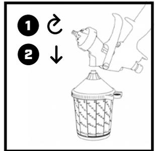
Remove the cup by gently twisting and pulling it off the adapter.
