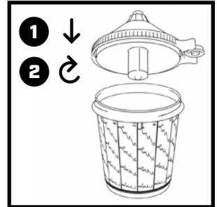
Screw the lid with the inserted sieve onto the cup.
