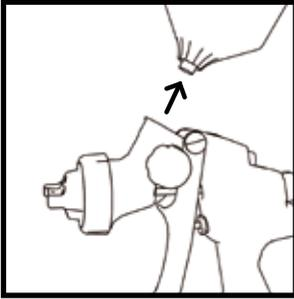
Remove the existing flow cup from the spray gun.
