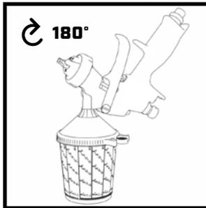
Turn the spray gun 180°. Briefly squeeze the trigger of the gun to drain the paint from the gun's color channel.
