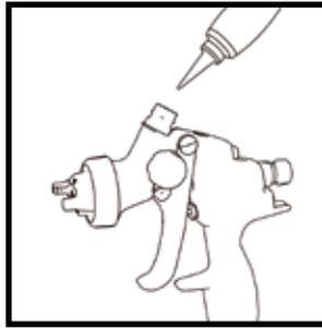
Operate the trigger while simultaneously supplying cleaning agent. Continue until cleaning is complete.
