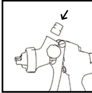
Attach the appropriate screw adapter to the spray gun (see adapter list).
