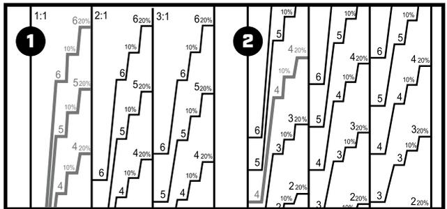
In each column, there are several stair-step gradations with identical numbers (1). Each of these gradations represents an independent mixing ratio (2).
